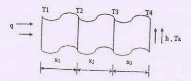
Calculate the temperature T1, T2, T3 and T4 assuming unit area of heat flow.
