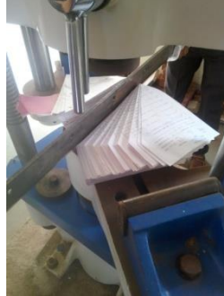
Fig.1 Force calculation on UTM machine. (It gives 10.54 kN of maximum force to cut paper of 40 mm thickness.)
