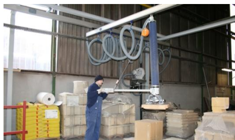
Fig 1.- Image showing lifting of solar panel using pneumatic gripper
