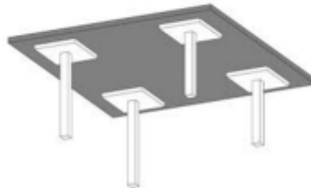
Fig -1: Typical shape of Reinforced Concrete Flat Slab with drop panel
